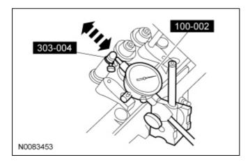
2. Move the Valve Guide Clearance Gauge toward the Dial Indicator Gauge with Holding Fixture and zero the Dial Indicator Gauge. Move the Valve Guide Clearance Gauge away from the Dial Indicator Gauge with Holding Fixture and note the reading. The reading will be DOUBLE the valve stem-to-valve guide clearance.
